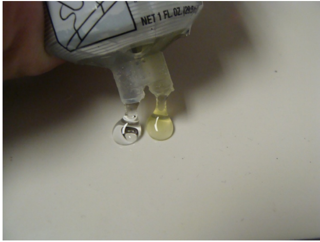
Fig 7. Dispense 2-part epoxy on clean surface.
