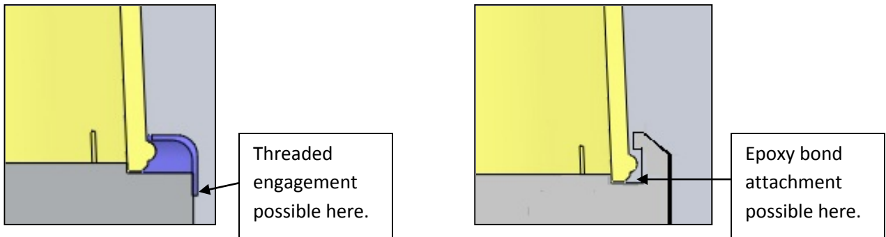
Fig 22. Attachment method and light loss
