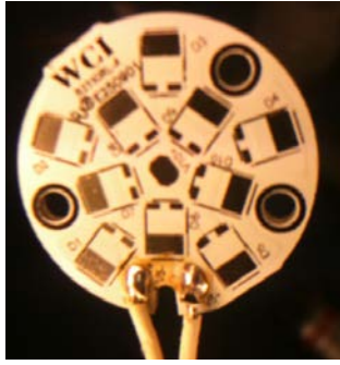
Fig 27. 10 LED PCB 22 gauge
