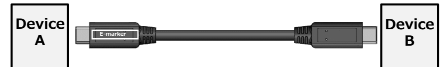
The E-Marker is incorporated in the cable assembly
